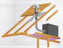
Make a quick connection from an attic furnace to a rigid B-Vent penetration.
