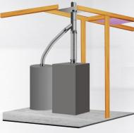
Make a direct connection from one or both appliances to a common B-Vent.
